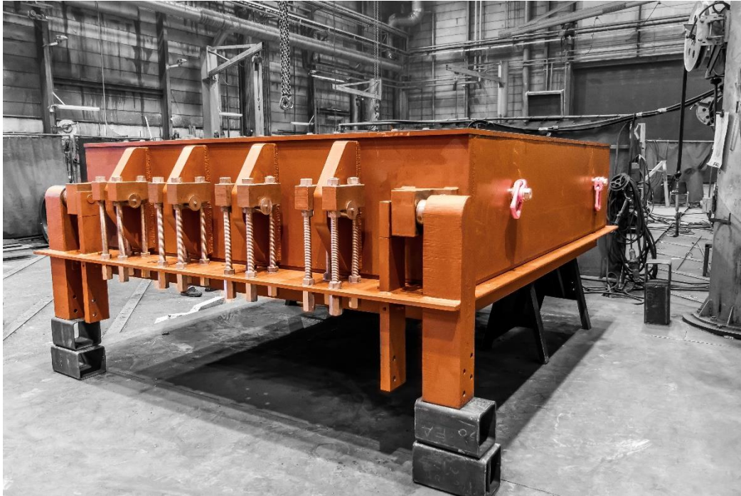
At the factory. Large (3m x 2,8m) single-leaf blast resistant steel door designed for 59 Bar (5900 kPa) / 11ms pressure-time load
